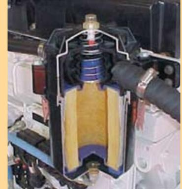
Cummins QSM11 marine engine with CCV cutaway
