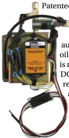
Patented Maintenance Systems DOC19 and DOC Plus will automatically change oil while the engine is running. The DOC19 systematically removes small amounts of oil from the engine, blends it into the return fuel line, and burns
