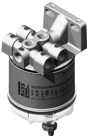
**All 600 Series Spin-On fuel filter/water separators feature multiple fuel ports (4 inlets and 3 outlets) and a unitized mounting bracket for installation convenience. Inlet and outlet threads are 3/8"-18 NPTF for all models. These filter assemblies provide flexibility during mounting and fit any engine application.**
