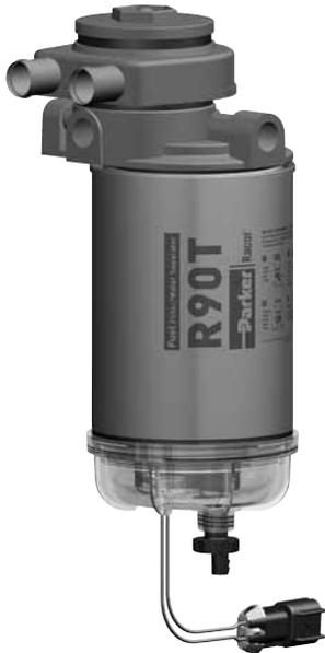
Racor's 300RC Series Fuel Filter/ Heater/Water Separators are specifically designed to handle today's tough fuel system problems. These units feature a standard high efficiency coolant heat exchanger to heat incoming fuel and are only different in flow capacity and element size.
