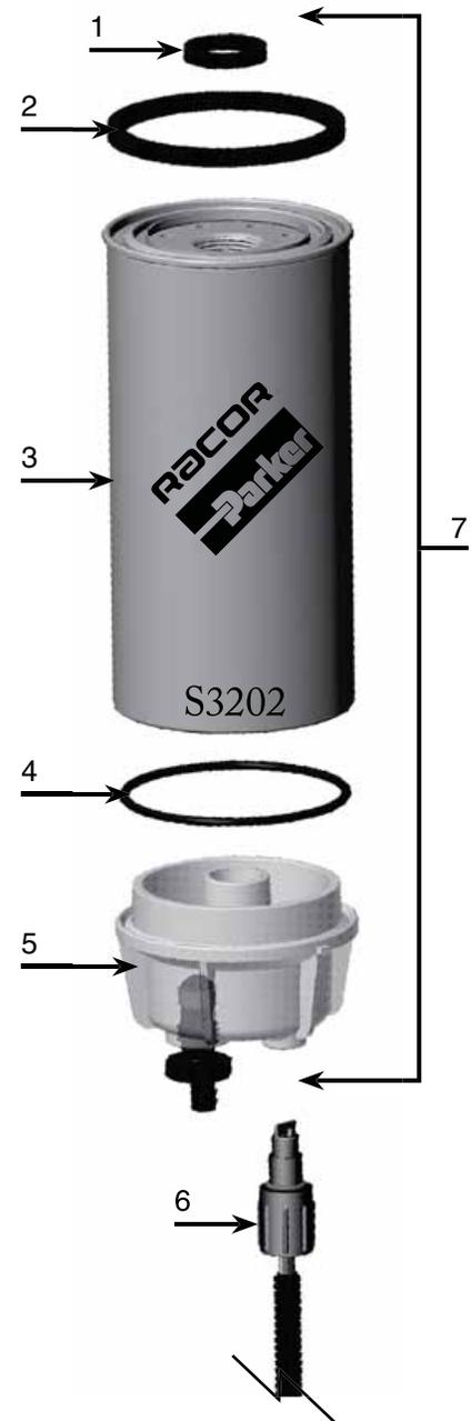
The standard B32002 bowl has no water sensor port. Bowls with water sensor ports are available as replacement kits (see item #5 above). Do not use water sensors on gasoline applications.
