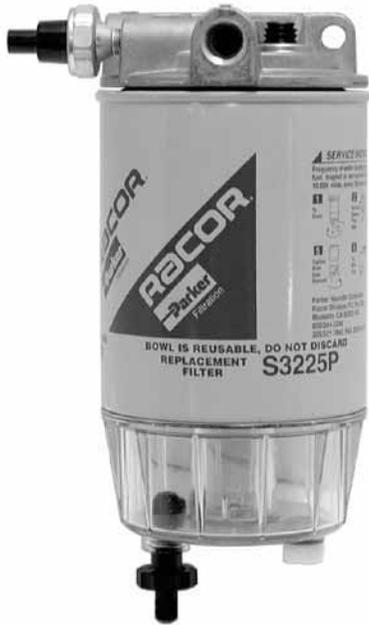
Racor's 325R Diesel Fuel Filter/ Heater/ Water Separators are specifically designed to handle today's tough fuel system problems. These units feature a standard in-head PTC heater and reusable see-thru contaminant collection bowl. They are different only in flow capacity and element size.
