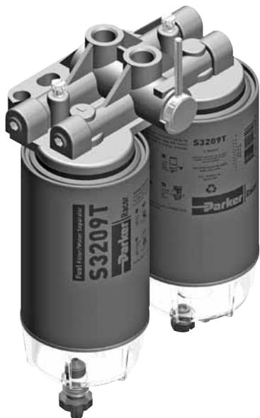
The Racor Dual Spin-On Series provides twice the filtering capacity in one compact and robust package. A shut-off valve located in the mounting head can switch to the clean filter so that the dirty filter may be serviced (servicing filters is not possible while engine is running).
