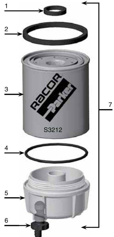
The standard B32012 bowl has no water sensor port. Bowls with water sensor ports are available as replacement kits (see item #5 above). Do not use water sensors on gasoline applications.
