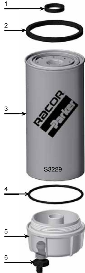
The standard B32029 bowl has no water sensor port. Bowls with water sensor ports are available as replacement kits (see item #5 above). Do not use water sensors on gasoline applications.
