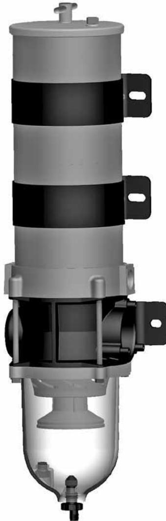
The electric primer kit can be retrofitted to many of the Racor 900 or 1000 series fuel filters already in service. The filter pump is an innovative and proprietary system consisting of a pre-screen filter, a flow bypass circuit and a roller cell pump powered by a 12 vdc motor or innovative 24 vdc Racor brushless motor.
