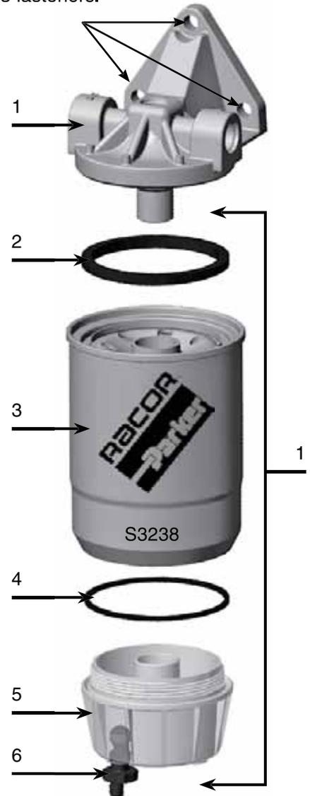
The standard B32038 bowl has no water sensor port. Bowls with water sensor ports are available as replacement kits (see item #5 above). Do not use water sensors on gasoline applications.
