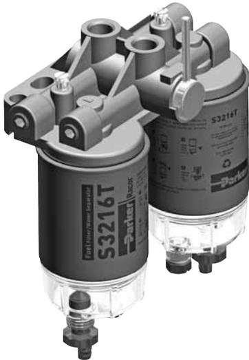
The Racor Dual Spin-On Series provides twice the filtering capacity in one compact and robust package. A shut-off valve located in the mounting head can switch to the clean filter so that the dirty filter may be serviced (servicing filters is not possible while engine is running).
