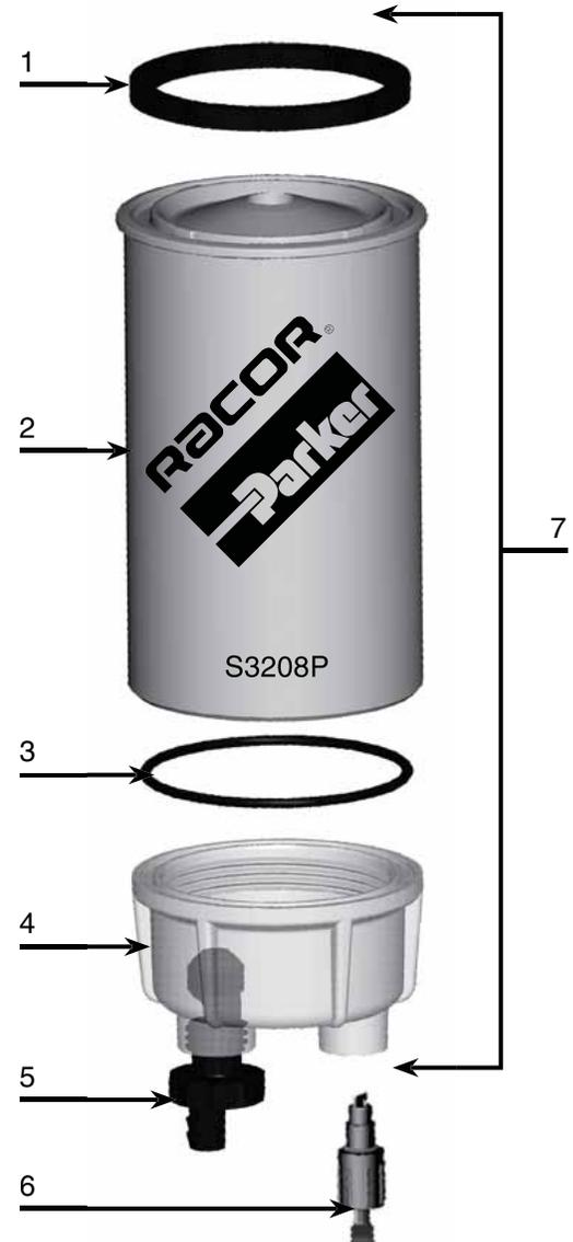
The standard B32008 bowl has no water sensor port. Other bowls with water sensor ports are available as replacement kits (see item #4 above). Water sensors are not for use with gasoline applications.
