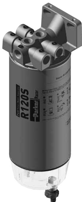
**All 600 Series Spin-On fuel filter/water separators feature multiple fuel ports (4 inlets and 3 outlets) and a unitized mounting bracket for installation convenience. Inlet and outlet threads are 3/8"-18 NPTF for all models. These filter assemblies provide flexibility during mounting and fit any engine application.**
